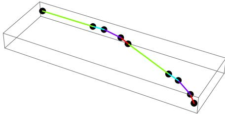
We rotate a backbone dihedral angle by certain degree. Only the tangent vectors with even index (corresponding to the inter-moiety bond) will be rotated.
