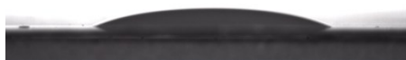
Fig. S2 The wettability of [VHIM][NTf 2 ] on SC treated AAO surface with CA of 18.57 \pm 0.42^\circ .
