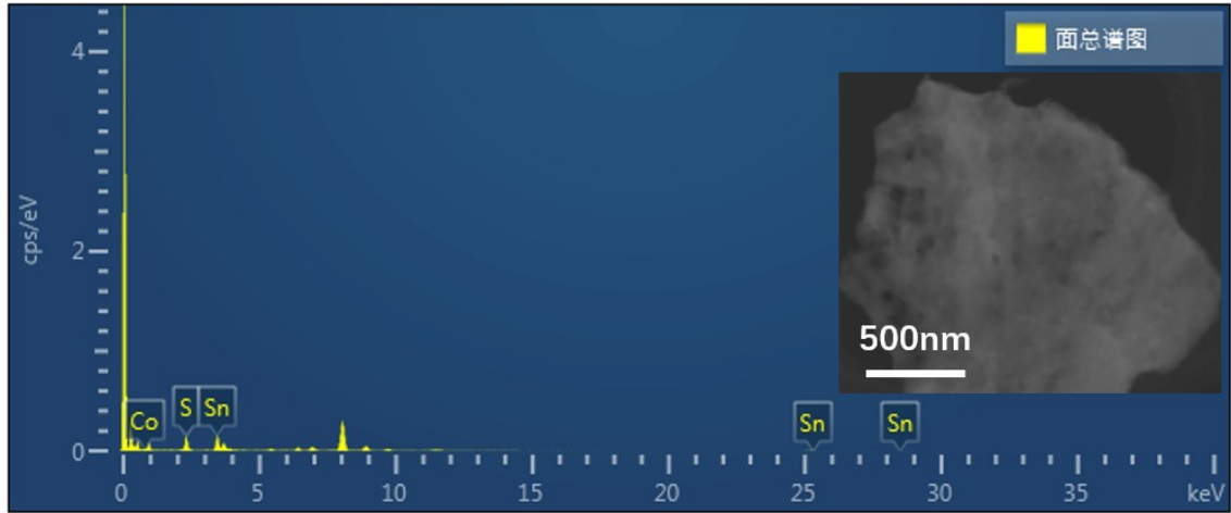
Fig. S3 The energy dispersive X-ray spectrum of the SnS 2 /Co 3 S 4 heterostructure nanosheets.
