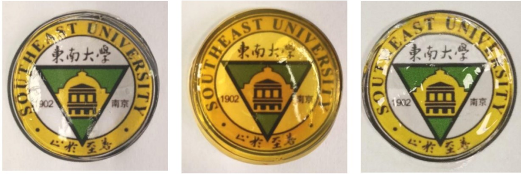
1 PAAm+Xg hydrogel PAAm-XgFe(III) hydrogel PAAm-XgFe(II) hydrogel 2 Figure S7. The light transmittance of the university badge covered with the PAAm+Xg (3% 3 w/v) hydrogel, the PAAm-XgFe(III)-3 hydrogel, or the PAAm-XgFe(II)-3 hydrogel. 4
