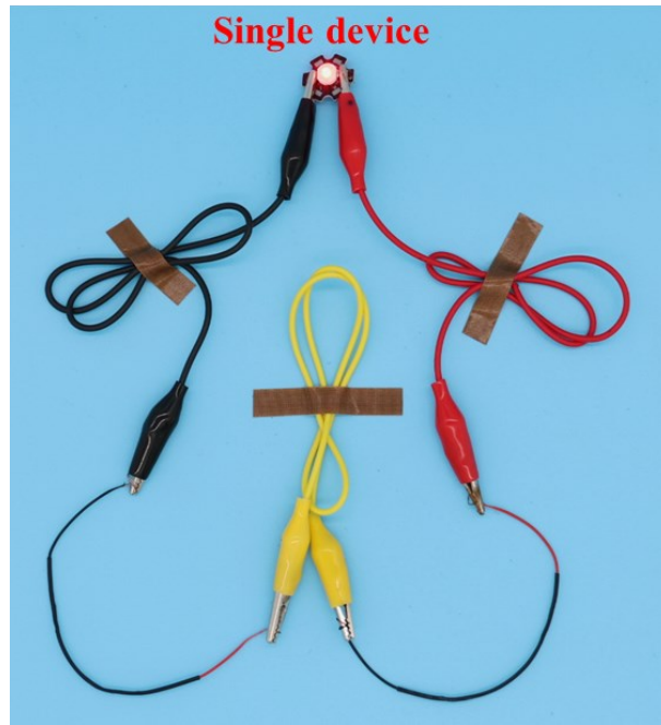
Figure S17. Photograph of a red LED illuminated by two single-devices.
