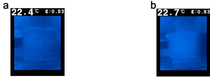
Fig.S14 Temperature of the fabric (a) before and (b) just after 1000 cycles of compression-and-decompression impacts (1 Hz, 13 N).
