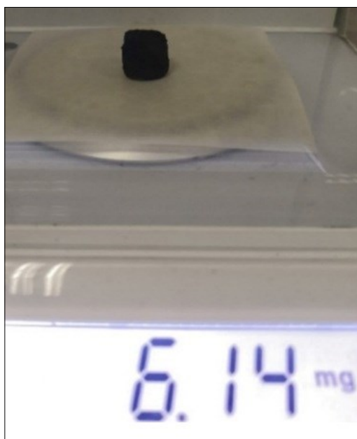
Fig. S3 Photographs of the as-prepared sample TOCF-800 weighting on an electronic balance, evidencing that the weight the sample is 6.14 mg. The diameter and height of sample TOCF-800 in cylinder configuration are 1.52 cm and 1.25 cm, respectively, demonstrating that its volume is \sim 2.27 \text{ cm}^3 . Accordingly, its density is ca. 2.7 \text{ mg cm}^{-3} .
