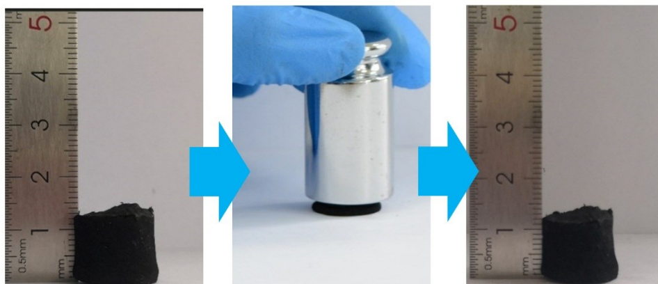
Fig. S4 The photographs to show one compression cycle over sample TOCF-800, representing its high flexibility.
