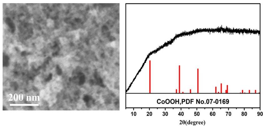
**Fig. S1** SEM and XRD of CoOOH INPs
