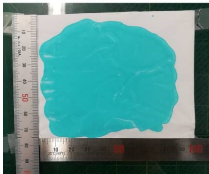
Figure S6. The digital photos of the CuBDC bulk coated Al 2 O 3 /PP separator.
