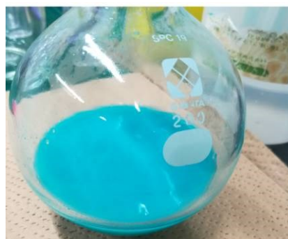
Figure S2. The CuBDC bulk solution prepared by using single solution method
