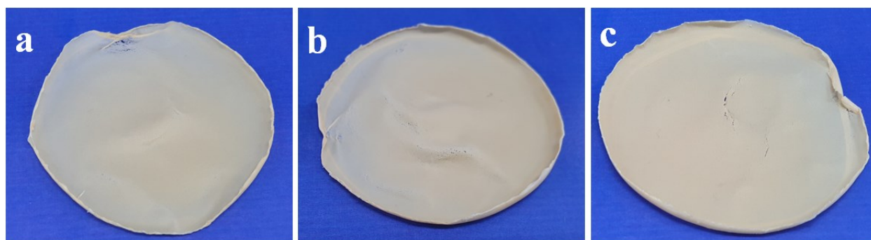
Fig. S8. Optical images of 5% MZ-CPE for ball-milling duration of (a) after 96 h, (b) after 144 h and (c) after 192 h.
