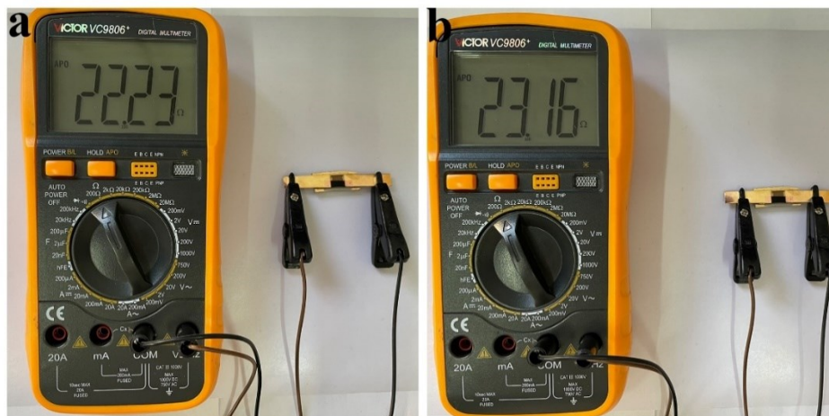
Fig. S9. (a) The resistance value of the rGO gradient wrinkled strain sensor. (b) The resistance value of the PRGW strain sensor.
