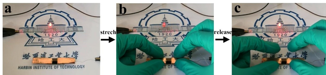
Fig. S14. Strain sensors are used to control the brightness of a LED lamp.
