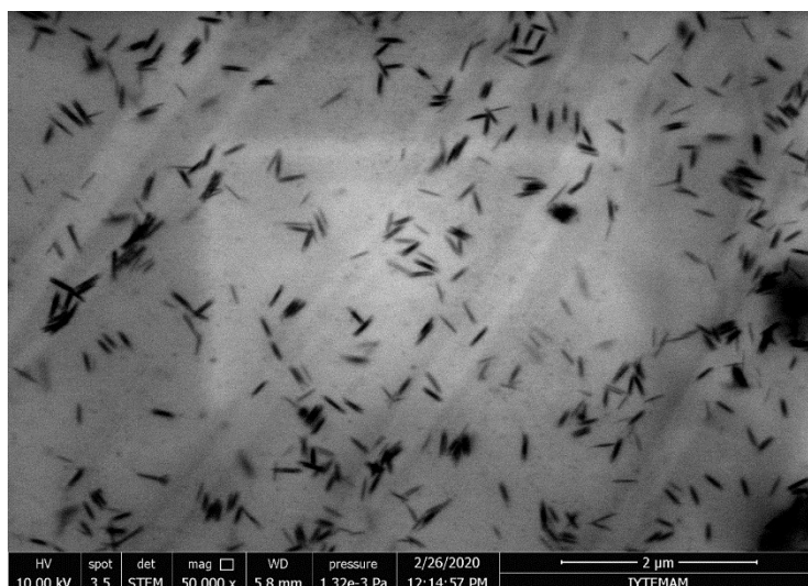
Fig. S1 Large area STEM image of halide perovskite nanoplatelets.
