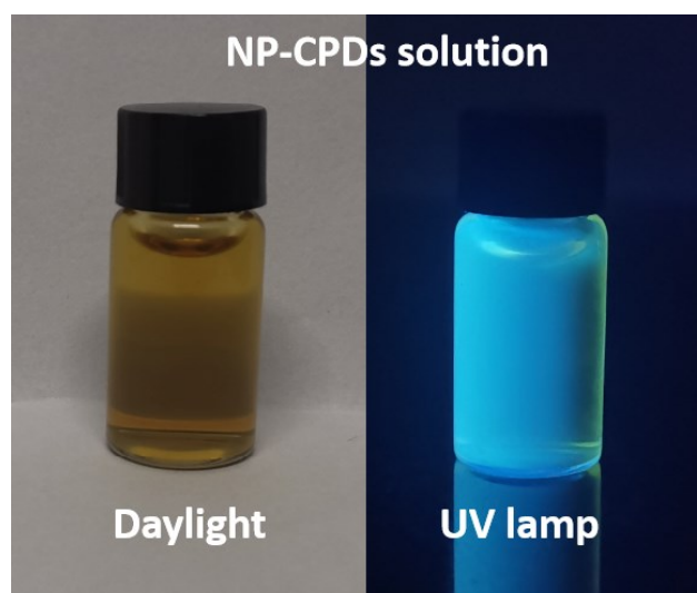
Fig. S8. Photographs of the NP-CPDs dispersion under daylight (left) and 365 nm UV lamp (right).
