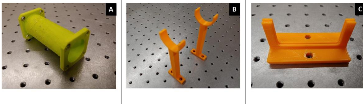
Figure S2 – 3D-printed assembly: A) Camera Tube. B) Camera Tube Supports. C) Flow Cell Holder.
