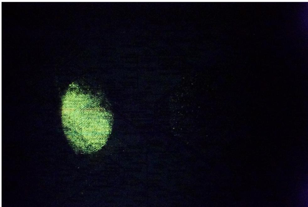
**Fig. S16:** Phosphorescent afterglow imaging showing only the 4-tpt powder.
