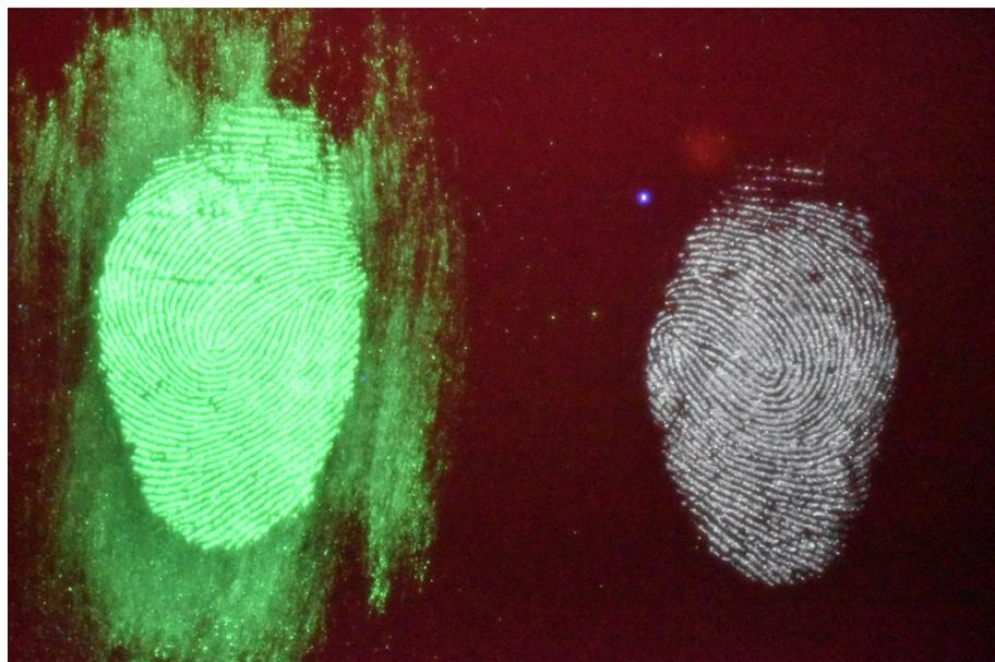
**Fig. S11:** Both commercial Fluro-Magnetic Print Powder (left) and doped 4-**tpt** powder (right) under UV Irradiation ( $\lambda = 365 \text{ nm}$ ). Surface is white tile.
