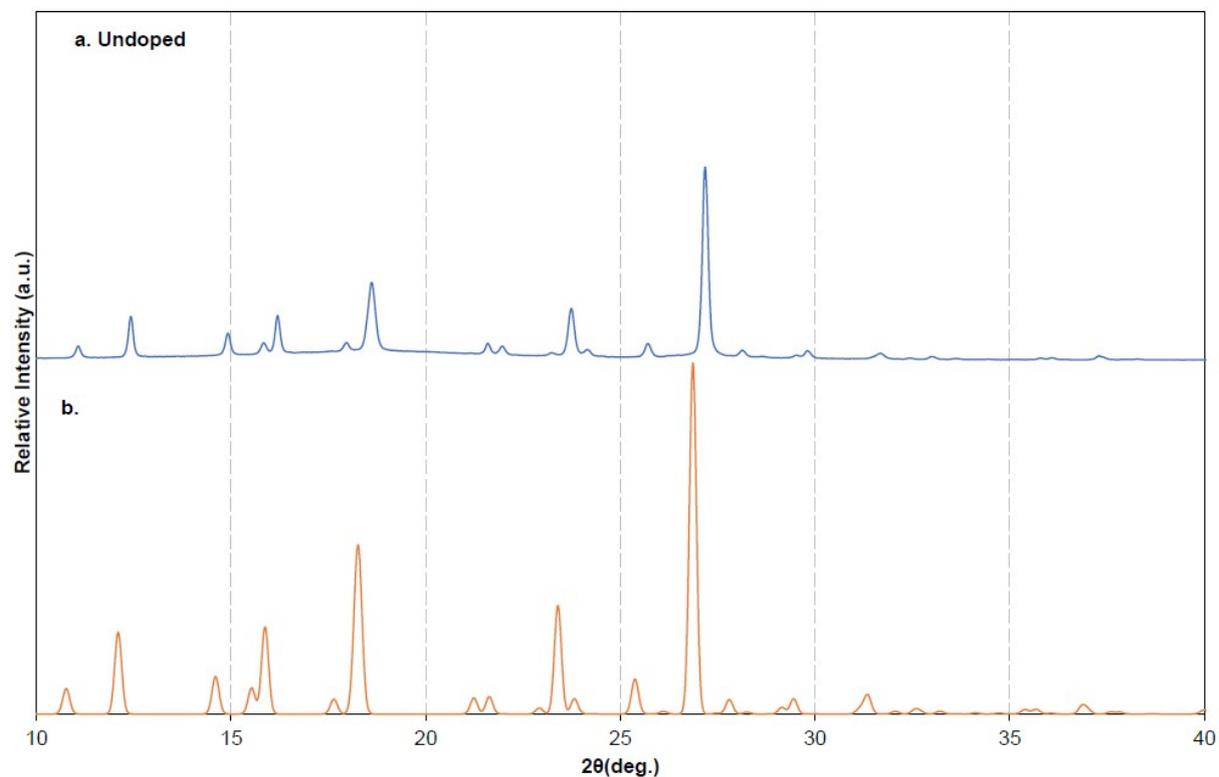
**Fig. S6:** Top (blue trace): undoped 4-tpt as-synthesised. Bottom (orange trace): the predicted PXRD pattern for the metastable form of tpt as reported in the literature.<sup>[2]</sup>
