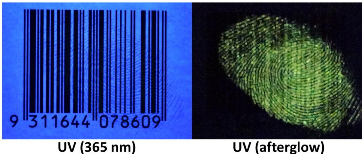
Fig. S13: Constant UV (left) and phosphorescent afterglow imaging (right). Note: only 4-tpt powder shown.
