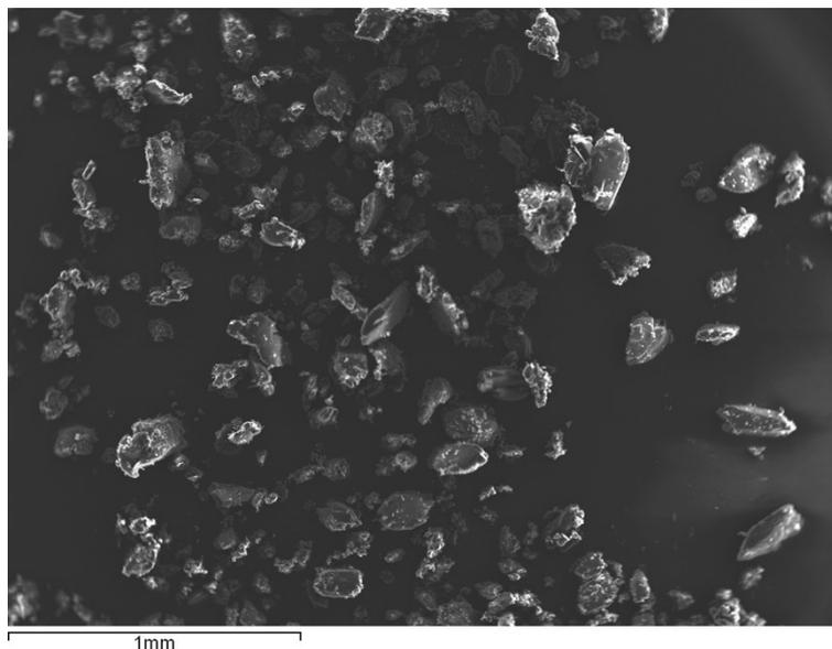
**Fig. S9:** A general cross-section of sizes for the as-synthesised doped 4-tpt. While a range of sizes are evident, an average particle diameter of 145  $\mu\text{m}$  can be inferred (see Fig. S10 for a representative enlargement).
