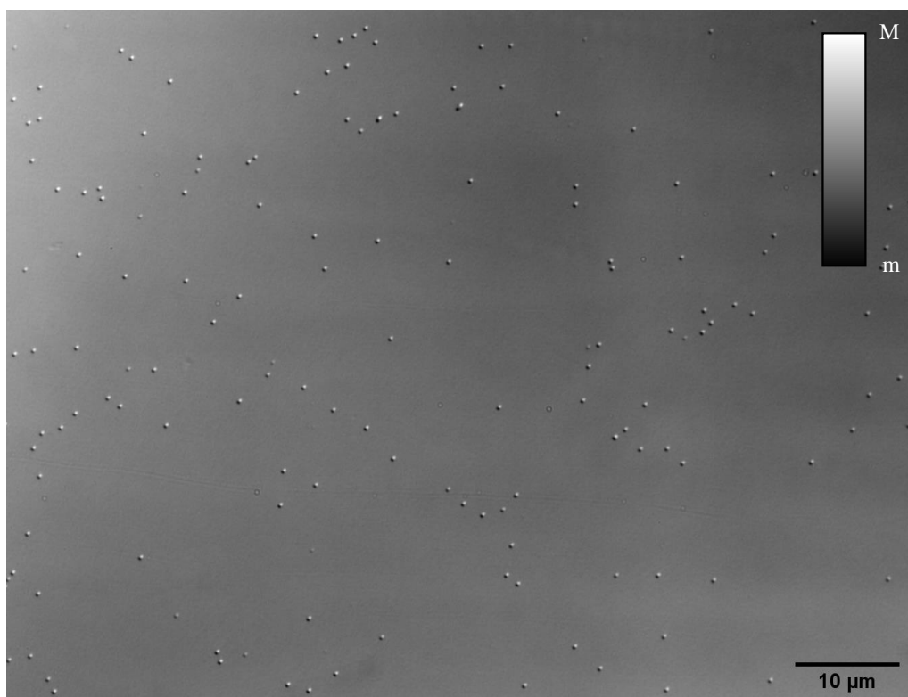
FIG. S7. I_+ image of the PS bead sample mounted in silicone oil ( m = 2600 to M = 3400 counts) at the same region shown in Fig. 1 imaged using the 1.45 NA objective and a phase offset of \psi = 30^\circ .
