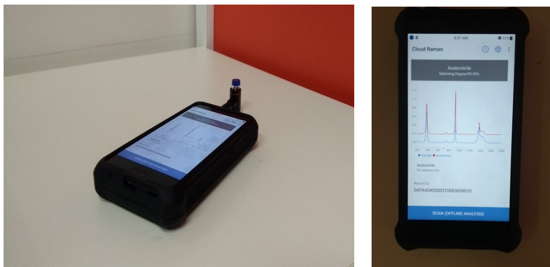
Fig. S1. Image of the Smart Raman XI TM with liquid vial holder
