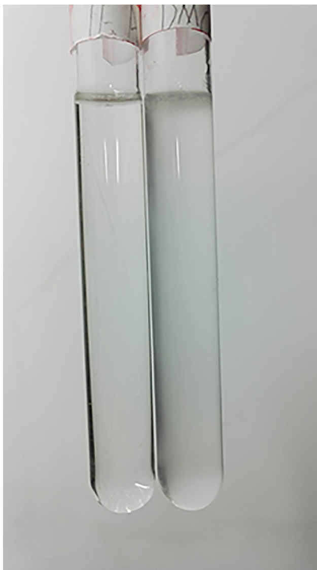
Fig. S1 Effect of SHS type on the extraction of 3 TFs. TEA on the left and DMCHA on the right. Extraction conditions: extraction solvent volume, 400 \mu L; ultrasonic time, 30 s; NaOH volume, 2 mL; NaCl, 0 g.
