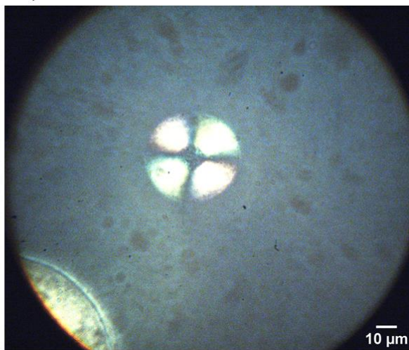
Fig. S1. Polarized light optical microscopy images of a) unlabeled and b) ThT-labelled spherulites with crossed polarizers.
