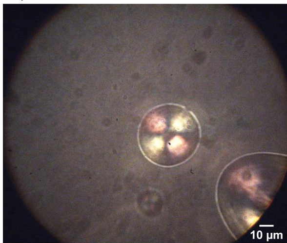
Fig. S1. Polarized light optical microscopy images of a) unlabeled and b) ThT-labelled spherulites with crossed polarizers.
