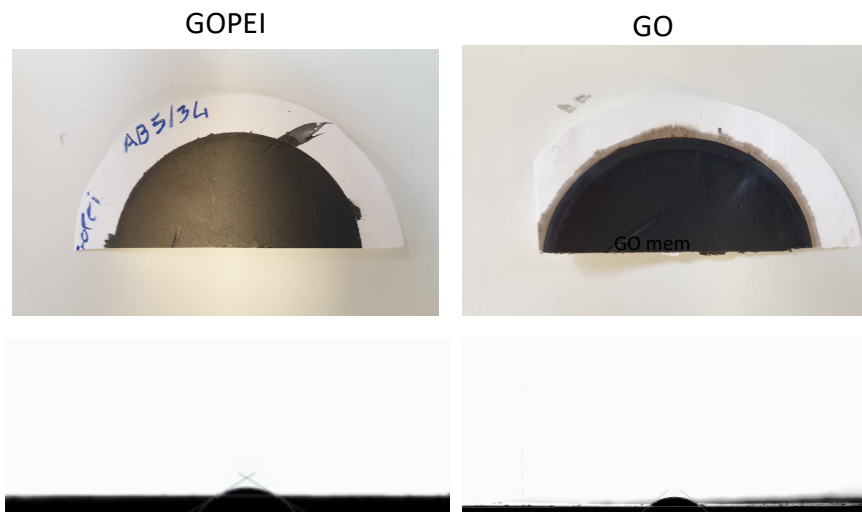
Figure S8. Top: membranes of GOPEI (left) and GO (right). Bottom: images of the water droplet on GO/GOPEI. GOPEI \theta=30.9^\circ , GO \theta=38.5^\circ .
