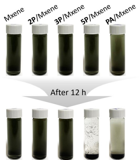
Fig. S6. The digital photos of pure and OPA modified Ti_3C_2T_x nanosheets suspensions after 12-h reaction.
