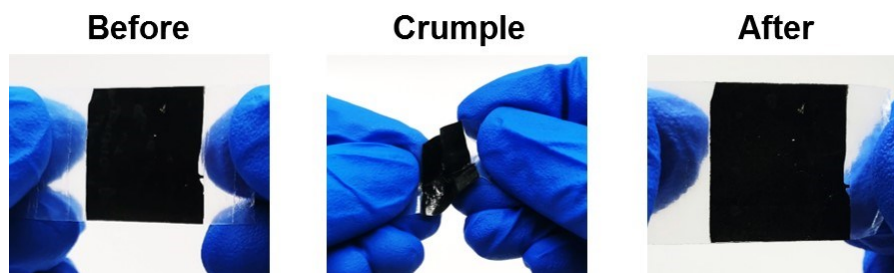
Figure S13. Photographs of the ultra-flexible and self-encapsulated devices (with the structure of PET/EVA/PET-PH1000/NiO x /Pervoskite/EVA/PCBM/PEI/PET-PH1000/PET/EVA) before and after crumpling test.
