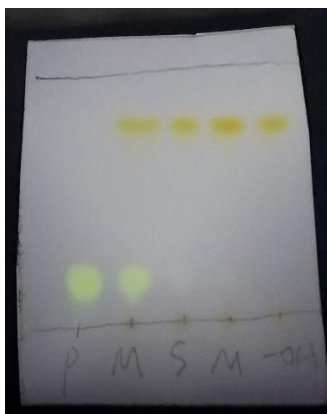
Figure S9. Photo of TLC plate for the reaction between DPP and \text{Cu}^{2+} under UV lamp (365 nm). From left spot to right one: DPP (spot P), DPP mixed with DPP-Cu 2+ system (spot M), DPP-Cu 2+ system (spot S), DHP mixed with DPP-Cu 2+ system (spot M), DHP (spot -OH). PE : EA = 3:2.
