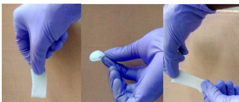
Figure S9. Photograph of foldable, bendable and stretchable nature of solid-state \text{NaVO}_3/\text{PAA}/\text{H}_2\text{SO}_4 electrolyte.
