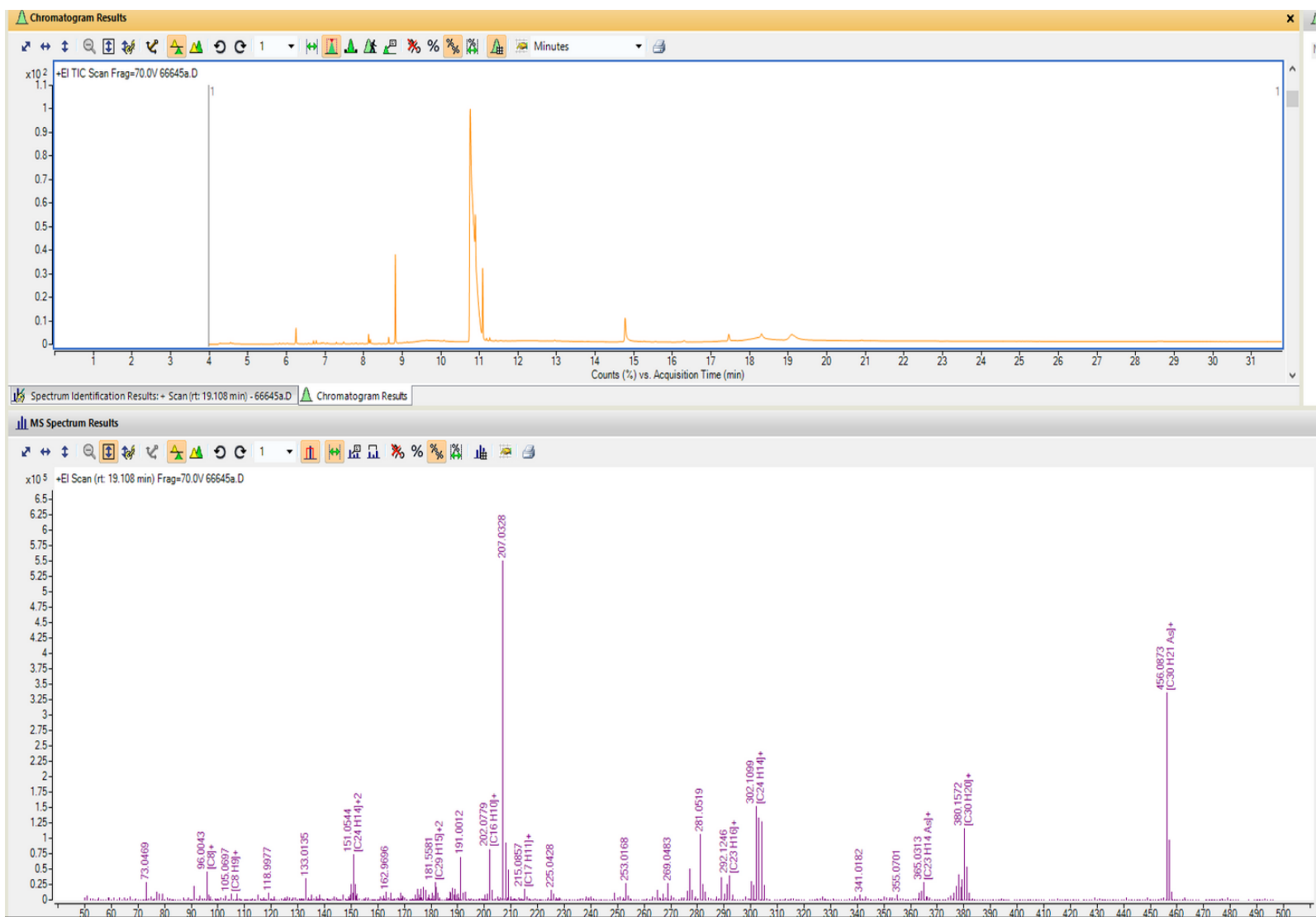
Figure S31. EI GC-MS of HC≡CAsC 4 Ph 4 (5)
