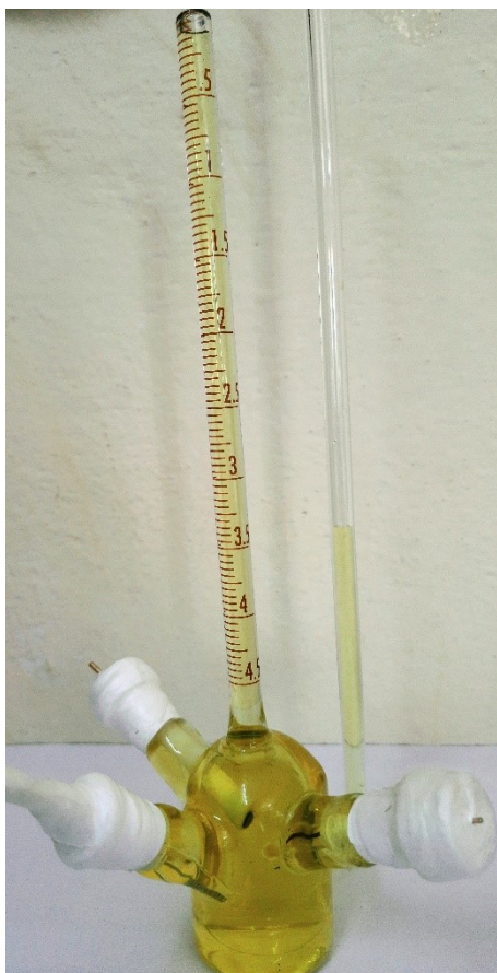
Fig. S33. Complete set-up of quantitative measurement of evolved H 2 gas by bulk electrolysis in three-electrode system consisting glassy carbon as working electrode, Ag/AgCl (3M) as reference electrode and platinum wire as counter electrode at current density of 1 mA/cm 2 .
