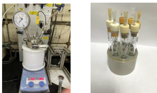
Figure S15. High-pressure steel autoclave and parallel reaction modulator.
