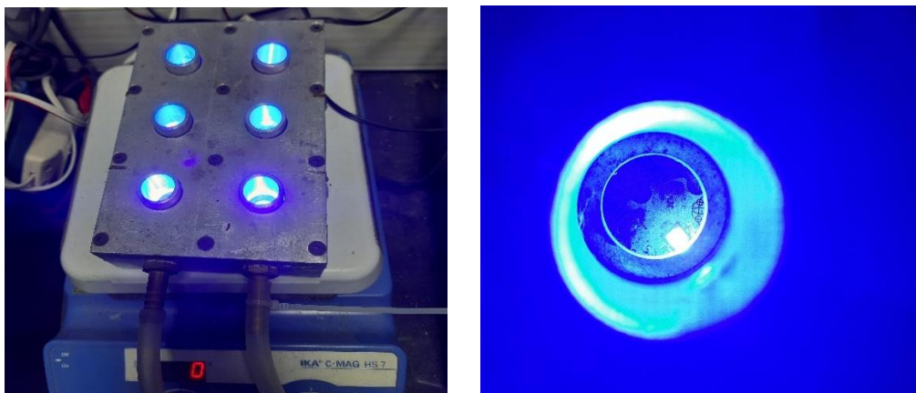
Figure S1: 3W blue LED photoreactor setup with magnetic stirring plate.
