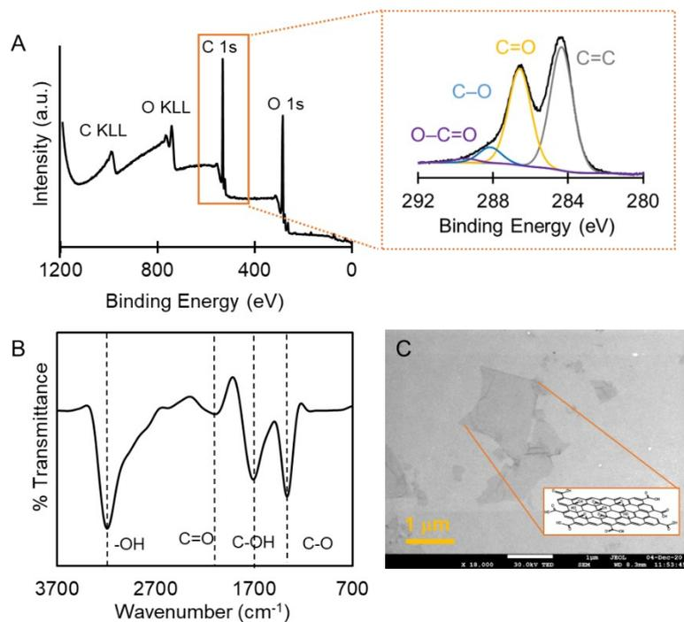
**Figure S1.** GONC characterization. A) X-ray photoelectron spectroscopy survey; Inset: C 1s X-ray photoelectron spectroscopy high-resolution spectrum; B) FT-IR spectrum; C) Scanning tunnel electron microscopy (STEM) micrograph.
