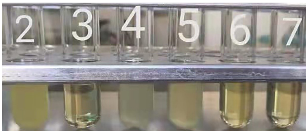
Fig. S18 Turbidity changes of S. aureus with Cu 2 O@CuO, Cu@Cu 2 S and antibiotics in test tubes: 2: Control; 3: Antibiotics; 4, 5: Cu 2 O@CuO; 6, 7: Cu@Cu 2 S
