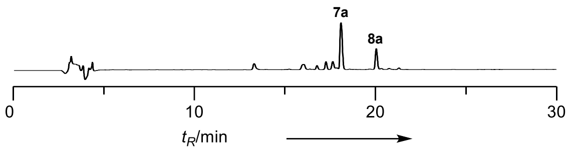
Fig. S5. Analytical HPLC chart of sequential intramolecular S–S and S–O acyl transfer reactions (reaction at 50 °C). Analytical HPLC conditions: linear gradient of solvent B in solvent A, 5% to 45% over 30 min.
