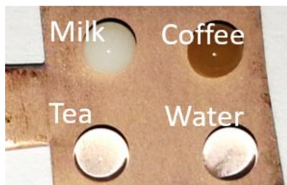
Figure S5. Photograph of various common liquid droplets in our daily life on the microflower-like superhydrophobic surface. indicating that the microflower-like surface possesses a strong resistance to the contaminant.
