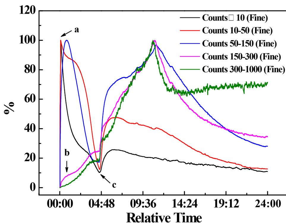
Fig S4. FBRM data monitor the crystallization of 5'-GMPNa<sub>2</sub> in Experiment 3. (a) the isopropanol solution were dropwise added to crystallizer.
