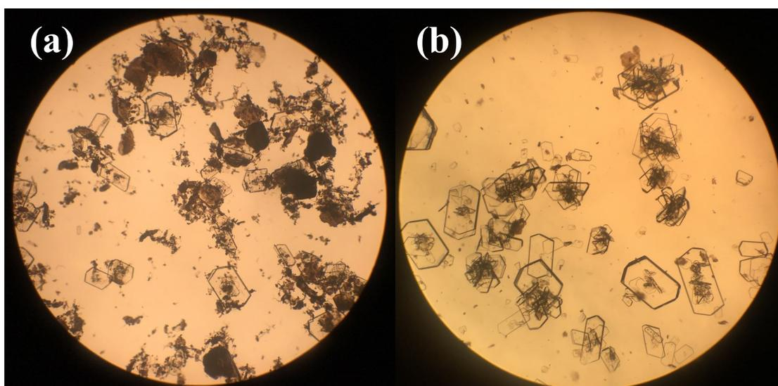
**Fig S5.** The process picture of crystallization Experiment 3 under a optical microscope ( $16 \times 4$ ). The morphology of solid in Experiment 3 at 8 h (a), at 24 h (b).
