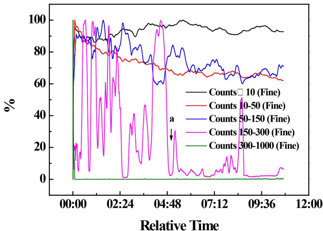
**Fig S3.** FBRM data monitor the crystallization of 5'-GMPNa<sub>2</sub> in Experiment 2. (a) the isopropanol solution were dropwise added to crystallizer.
