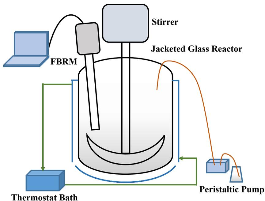
Fig. S1. Experimental device diagram of oiling-out process monitoring and control.
