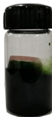
Figure S6. (a) Experimental device diagram of chemical prelithiation; (b) Photo of Lithium-4,4'-Dimethylbiphenyl reagent (1 M Li-4,4'-DMBP)
