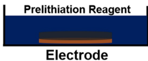
Figure S6. (a) Experimental device diagram of chemical prelithiation; (b) Photo of Lithium-4,4'-Dimethylbiphenyl reagent (1 M Li-4,4'-DMBP)
