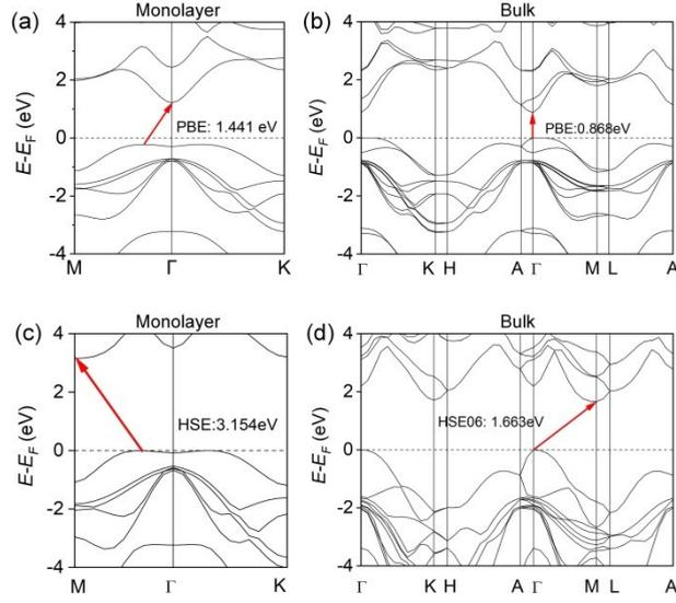
**Fig. S1** The band structure of monolayer and bulk InSe using (a-b) PBE and (c-d) HSE06 approaches. Blue rectangle illustrates two pairs of doubly degenerate valence bands of monolayer InSe.
