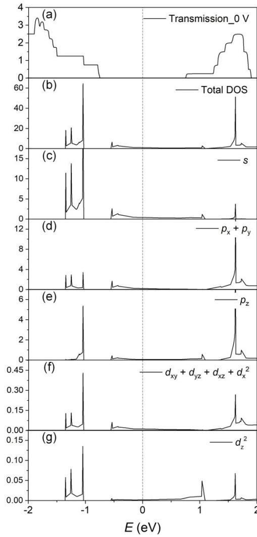
**Fig. S2** (a) The transmission coefficient as a function of electron energy in the armchair direction of monolayer InSe photodetector at 0 V. (b) The total density of state and (c-g) partial density of state of monolayer InSe.
