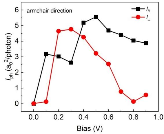
**Fig. S3** The variation in  $I_{ph}$  with the source-drain bias voltage of monolayer InSe in the armchair direction.
