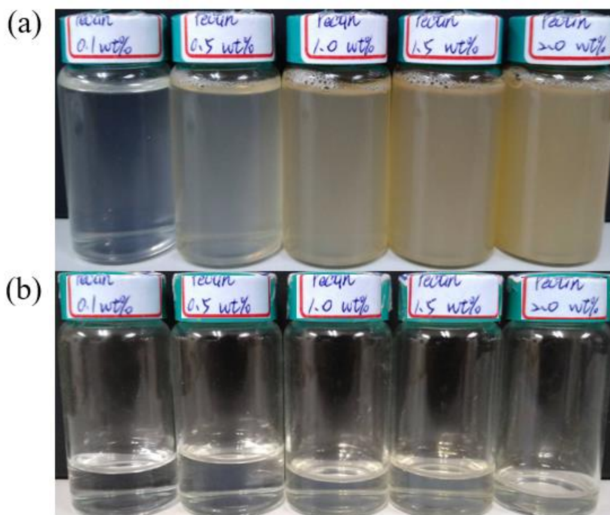
Fig. S2 Photographs showing the outer appearance of (a) the original and (b) filtered pectin solutions at various concentrations: 0.1, 0.5, 1.0, 1.5, and 2.0 wt.%.
