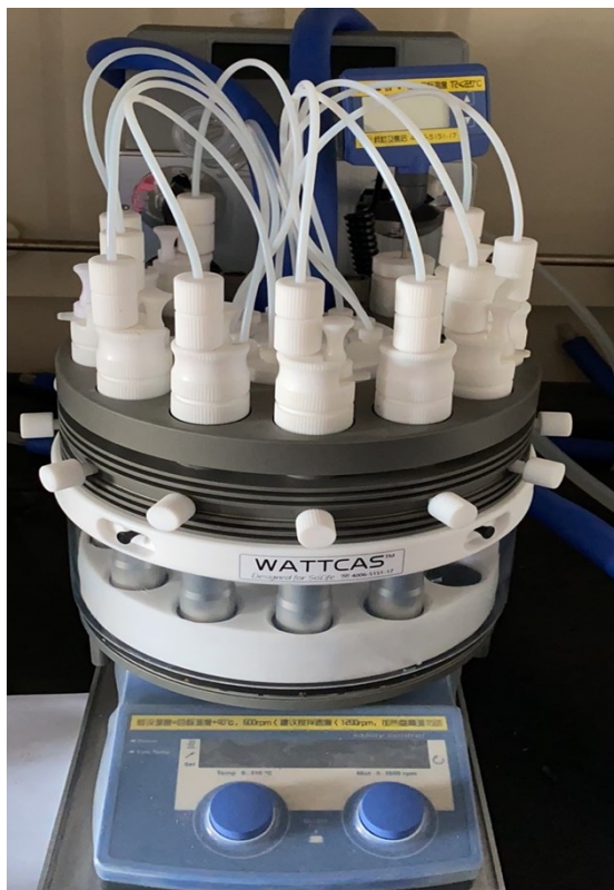
Fig. S5 WP-TEC-1020HSL photochemical reaction system.
