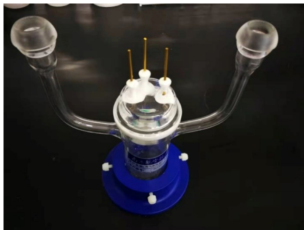
Figure S2 The image of high gas tightness single chamber three electrode reactor.
