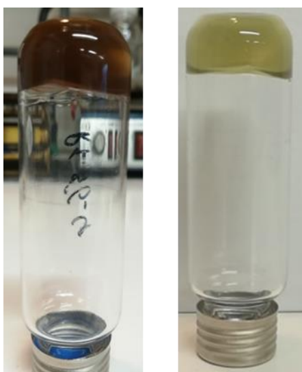
Figure S50 – Crosslinked silicones by \text{Co}(\text{tmhd})_2 before prolonged air ( \text{O}_2 and moisture) contact (left) and after (right)
