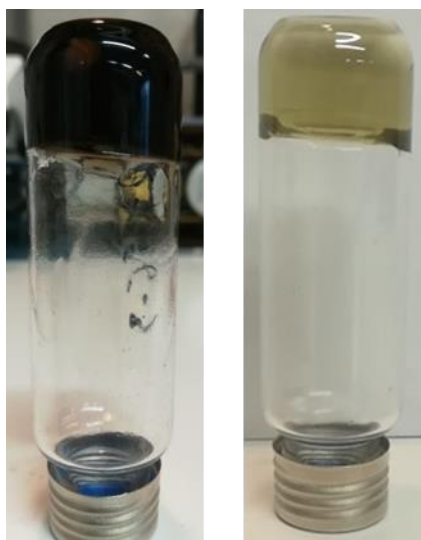
Figure S49 – Crosslinked silicones by \text{Co}(\text{acac})_2 before prolonged air ( \text{O}_2 and moisture) contact (left) and after (right)
