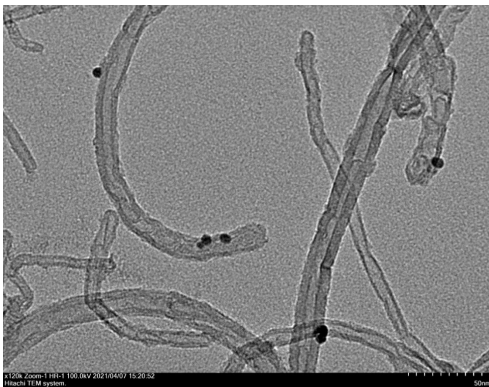
Figure S27. TEM images of Pt nanoparticles of Pt/MWCNT THF after the model reaction.
