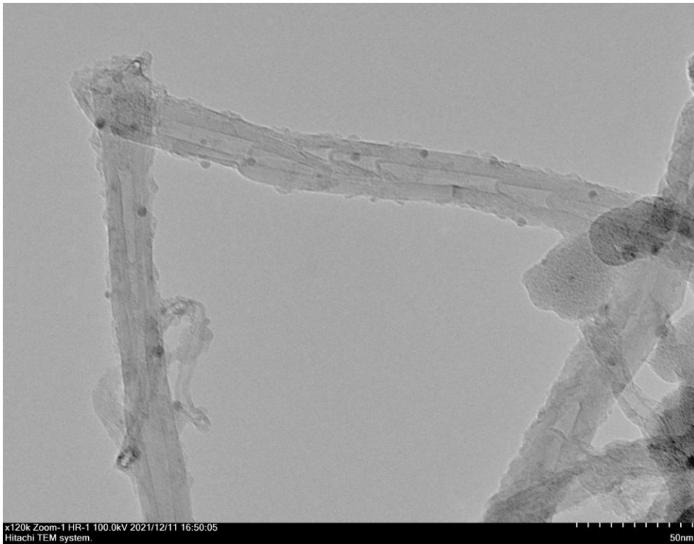
Figure S29. TEM images of Pt nanoparticles of Pt/MWCNT THF after allyl bromide hydrosilylation by HSiCl 3 .
