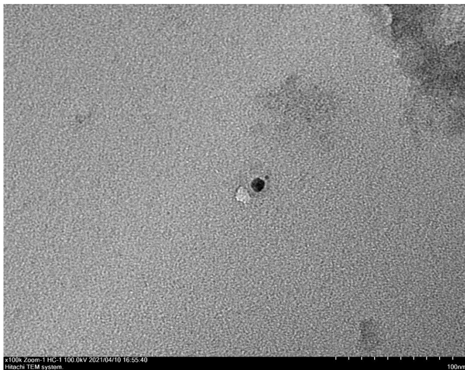
Figure S31. TEM image of Pt NPs from HSiCl 3 ( 2a ) and Ph 2 C 2 ( 1a ) reaction supernatant in the presence of Pt/MWCNT THF .
