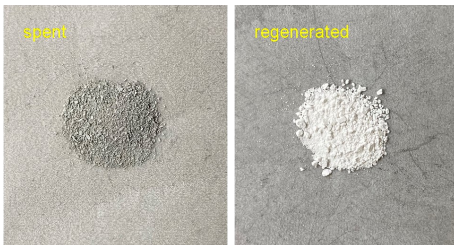
Fig. S11. Appearance images of the spent and regenerated Y-Zn 0.02 Zr 0.02 /Si-beta catalyst.
