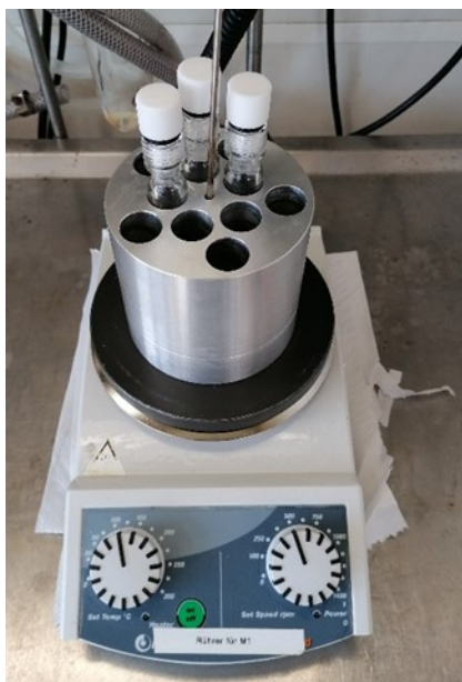
Figure S1: steel block and pressure tubes on stirrer/heating plate
