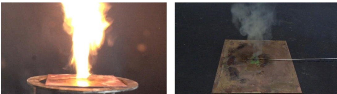
Figure S36. Deflagration of the picrate complex 17 during hot plate test (left) and decomposition during hot needle test (right).
