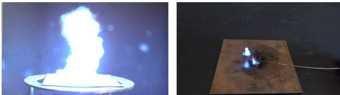
Figure S31. Reaction of the coordination compound 11 during hot plate (left) and hot needle test (right).
