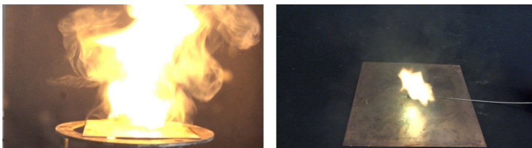
Figure S41. Results of hot plate (left) and hot needle test (right) of the styphnate coordination compound 21 .
