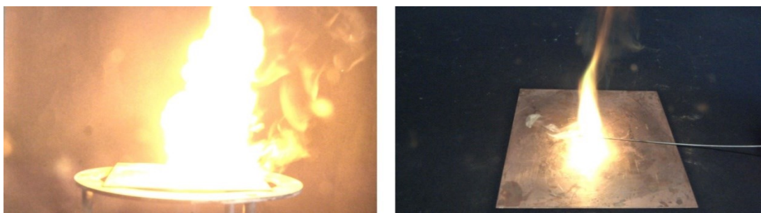
Figure S40. Deflagration of the picrate complex 20 during hot plate test (left) and hot needle tests (right).
