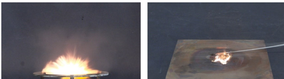
Figure S33. Detonations of the copper azide complex 14 during hot plate (left) and hot needle test (right).
