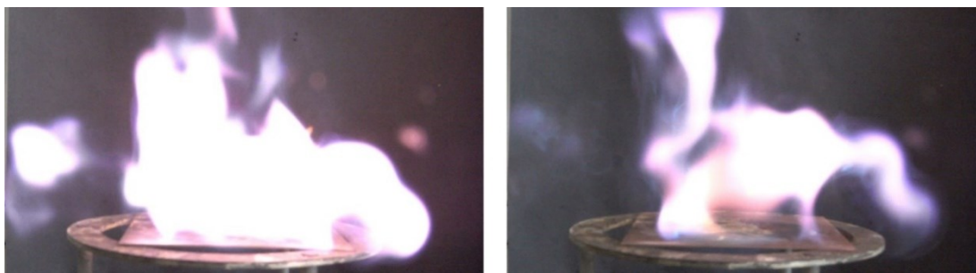
Figure S30. Deflagration of the zinc chlorate complex 9 during hot plate test.
