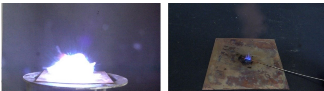
Figure S29. Deflagration reaction of ECC 8 during hot plate (left) and hot needle test (right).
