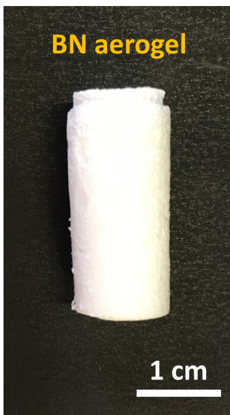
Fig. S3 A digital photo of a BN aerogel prepared in a centrifuge tube.
