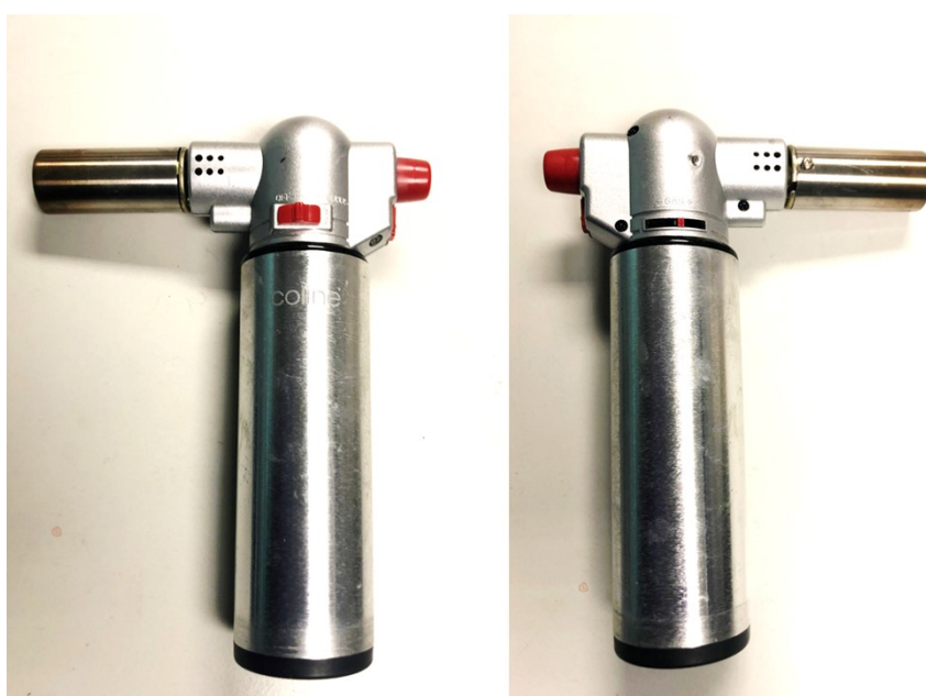
Fig. S10 Digital photo of the blow torch used for burning BN aerogels.
