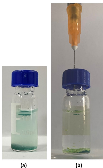
Fig. S4 (a) The samples of compound Gd 22 Ni 21 immersed in water; (b) The samples of compound Gd 22 Ni 21 immersed in water with concentrated H 2 SO 4 (80 μL).
