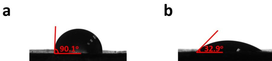
**Figure S12.** Contact angle images of the (a) as prepared Cu-Si@C electrode and (b) the Cu-Si@C electrode after discharge.
