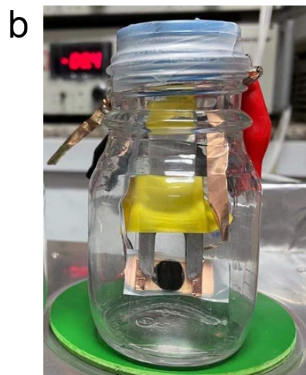
Fig. S23 (a) Device for photo-assisted lithium-ion battery. (b) Home-made lithium-ion battery.
