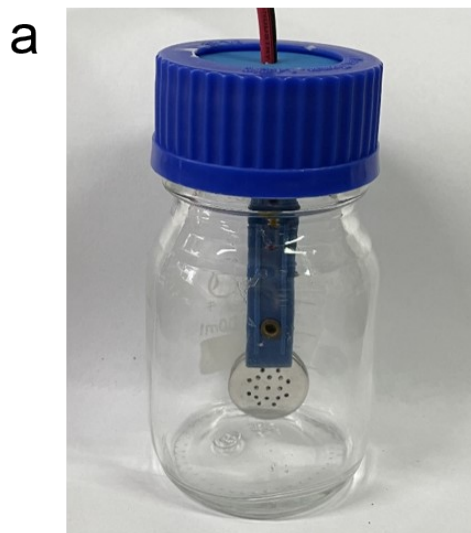
Fig. S23 (a) Device for photo-assisted lithium-ion battery. (b) Home-made lithium-ion battery.
