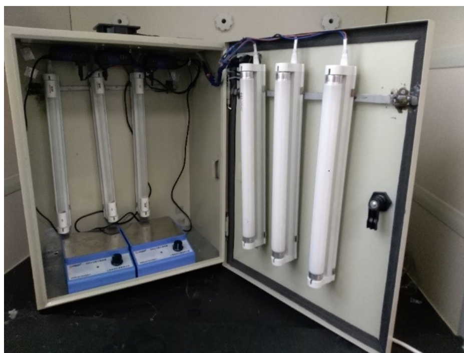
Figure S7 Reactor for disinfection and photoreactivation
