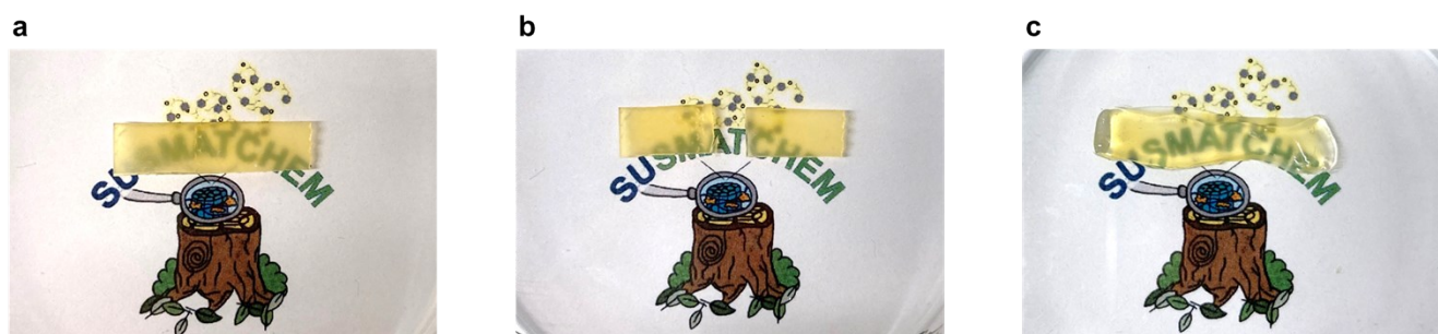
Figure S12. (a) PBMA-GOx-chi-LNPs 10 composite film. (b) PBMA-Gox-chi-LNPs 10 film after tensile test. (c) PBMA-GOx-chi-LNPs 10 composite film after recycling by melting process from specimen displayed in b.
