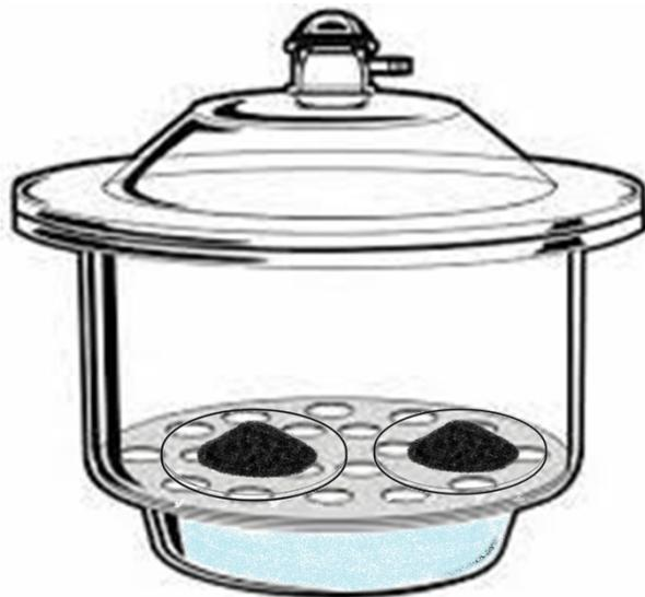
**Fig. S8** Improvised humidifier using a desiccator containing water at the bottom and the samples on the glass disc.
